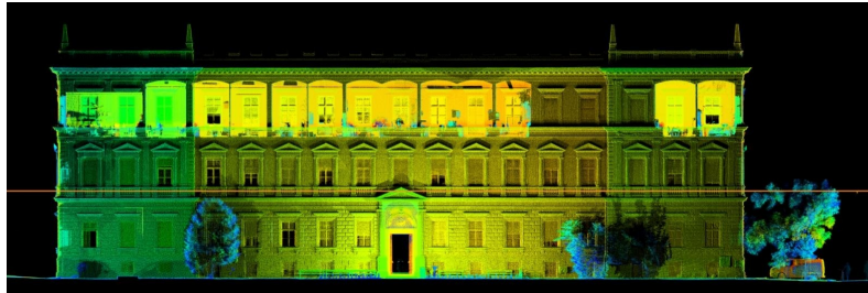
Figure 2.1: High-resolution point cloud of a terrestrial laser scan. The colors indicate the reflectivity of the individual surfaces and textures. The reflectivity is determined by the intensity and shape of the return pulse. (Skyability GmbH (2021))
